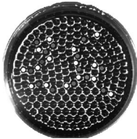
FIGURE 1. Penta–hepta defects represented by pairs of white and grey dots. The hexagonal pattern contains lines of defects that form grain boundaries. Several hexagonal patterns with different orientations in the container are observed.
